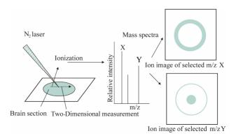
**Figure 1.** Schematic illustration of imaging mass spectrometry (IMS).
